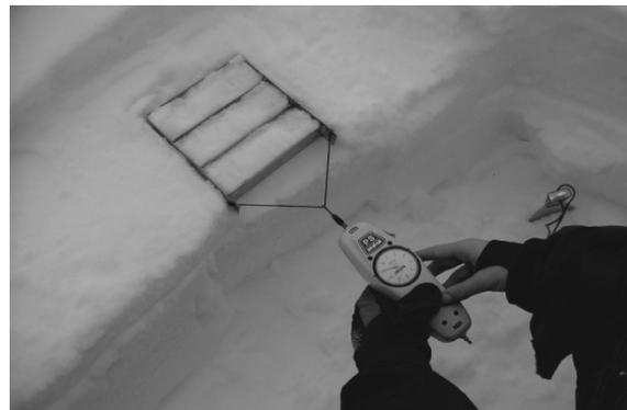
Figure 1 – Shear Frame Test
