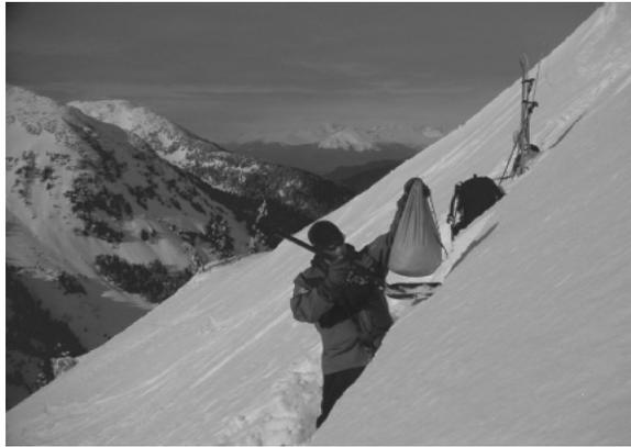
Figure 2 – Conducting a Stuffblock Test at Eaglecrest
